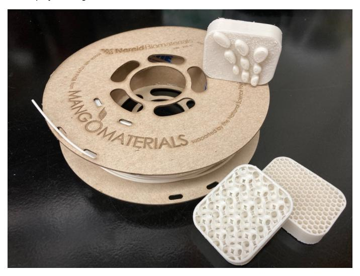
Examples of Nereid's early prototypes: A reel of PHB made from Mango Materials' bioplastic pellets, next to some 3-D printed parts
