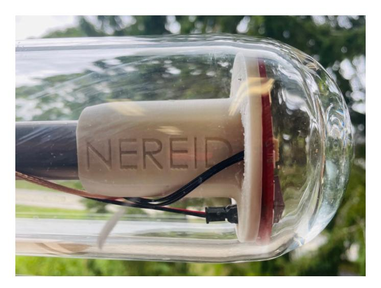
The first ocean instrument made with 3D-printed internals produced by the Nereid Biomaterials team
