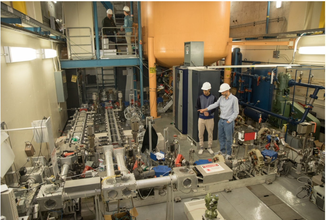
Mark Sherwin (bottom right) explains the inner workings of the free-electron laser. The large yellow tank accelerates electrons, which are guided along the beam line
