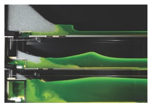
A photograph of an experimental lab setup reflecting the fluid dynamics of a tsunami
