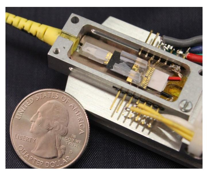
The internal workings of the turnkey soliton microcomb chip, with quarter for scale.
