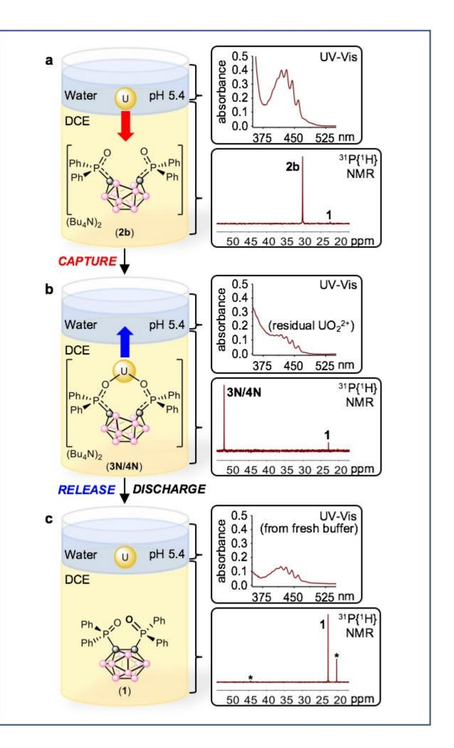
An illustration of the electrochemical switching method to capture and release uranium ions
