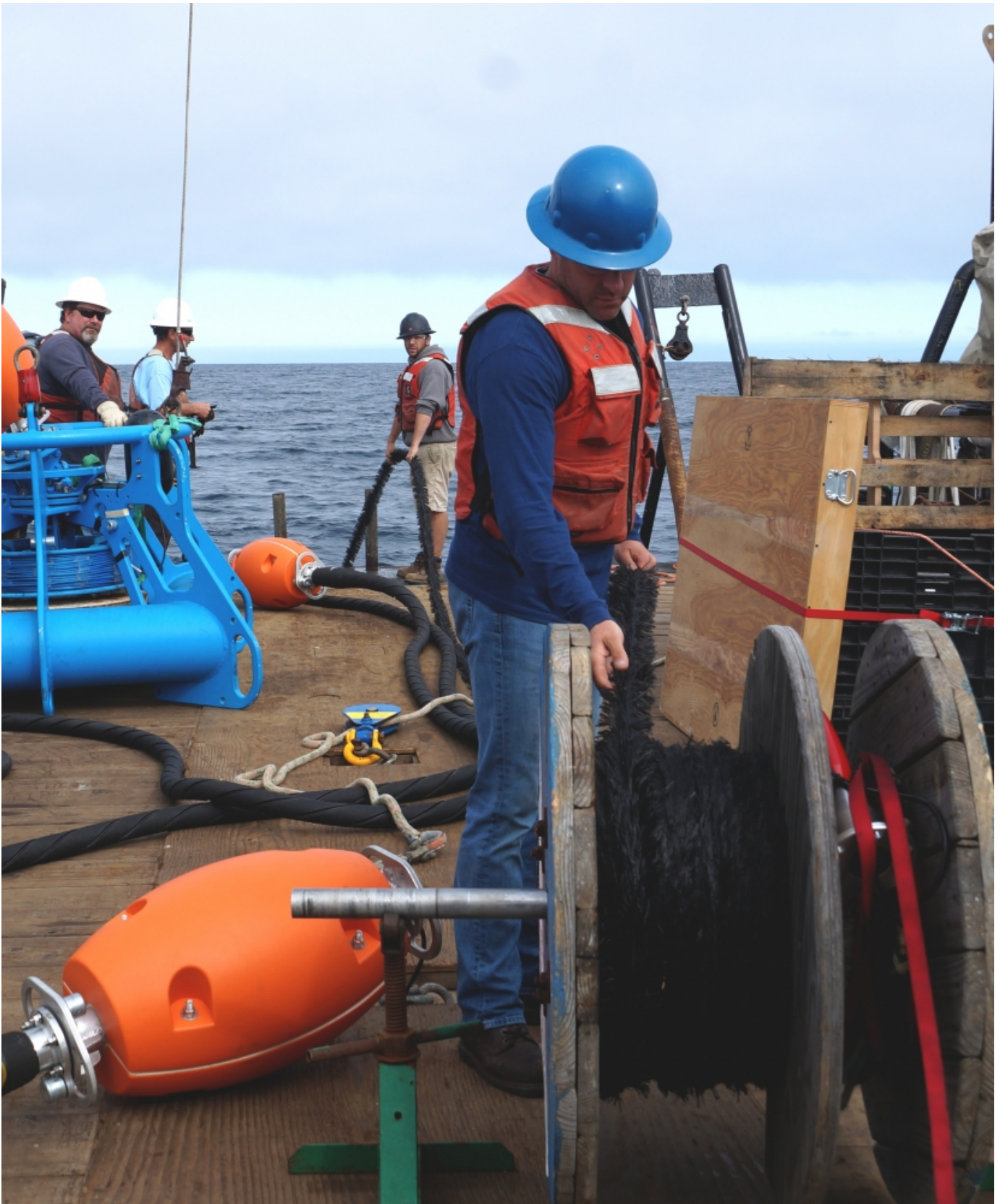
A segment of the line is covered in a "furry" cladding to attenuate vibration. Credit: Sonia Fernandez
